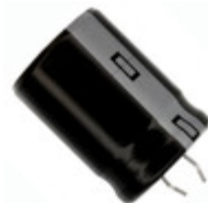
ECO-S1JA102BA Panasonic Electronic Components CAP ALUM 1000UF 20% 63V SNAP
