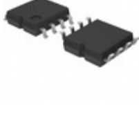
BR25H020F-2LBH2 LAPIS Semiconductor IC EEPROM 2K SPI 10MHZ 8SOP
