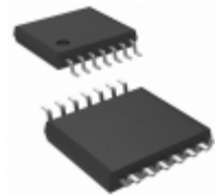
AD8624ARUZ-RL Analog Devices Inc. IC OPAMP VFB 560KHZ RRO 14TSSOP
