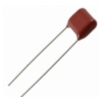
ECQ-E6273KF Panasonic Electronic Components CAP FILM 0.027UF 10% 630VDC RAD
