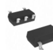
S-80138BLMC-JEXT2U SII Semiconductor Corporation IC VOLT DETECTOR 3.8V SOT23-5
