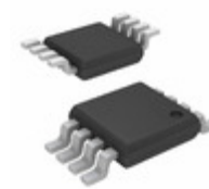
MIC5208-3.8BMM-TR Microchip Technology IC REG LDO 3.8V 50MA 8MSOP
