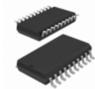
MC68HRC98JK3ECDW NXP USA Inc. IC MCU 8BIT 4KB FLASH 20SOIC
