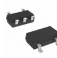
S-1167B28-M5T1G SII Semiconductor Corporation IC REG LDO 2.8V 0.15A SOT23-5
