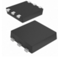
S-1167B29-I6T2G SII Semiconductor Corporation IC REG LDO 2.9V 0.15A SNT6A
