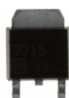
AN7715SP Panasonic Electronic Components IC REG LDO 15V 1.2A SP3SUA
