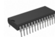
AT28C256-15PC Microchip Technology IC EEPROM 256KBIT 150NS 28DIP
