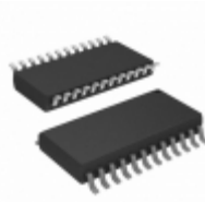
AD7228KRZ Analog Devices Inc. IC DAC 8BIT OCTAL W/AMP 24SOIC
