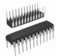
AD7228KNZ Analog Devices Inc. IC DAC 8BIT OCTAL W/AMP 24-DIP
