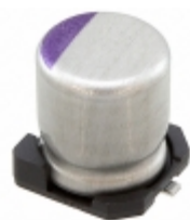
2R5SVPB120M Panasonic CAP ALUM POLY 120UF 20% 2.5V SMD
