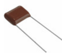
ECQ-E4394RJF Panasonic Electronic Components CAP FILM 0.39UF 5% 400VDC RADIAL
