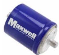
BCAP1200 P270 K04 Maxwell Technologies Inc. CAP 1200F 2.7V THREADED
