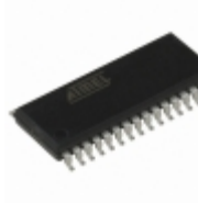
AT28C010-20SI Microchip Technology IC EEPROM 1MBIT 200NS 32SOIC
