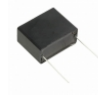
ECQ-UAAF225K Panasonic Electronic Components CAP FILM 2.2UF 10% 275VAC RADIAL
