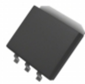
MIC37300-1.5BR Microchip Technology IC REG LDO 1.5V 3A SPAK-3
