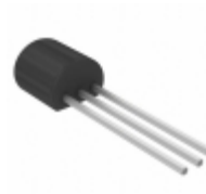
AN78L15 Panasonic Electronic Components IC REG LDO 15V 0.1A 3SSIP
