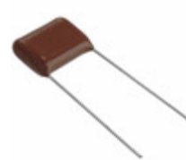
ECQ-E1225JF3 Panasonic Electronic Components CAP FILM 2.2UF 5% 100VDC RADIAL
