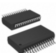
PIC18LF27K40T-I/SS Micrel / Microchip Technology IC MCU 8BIT 128KB FLASH 28SSOP
