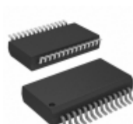
PIC18LF27K40-E/SS Micrel / Microchip Technology IC MCU 8BIT 128KB FLASH 28SSOP
