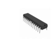
**UDN2916B-T** Allegro MicroSystems, LLC IC MOTOR DRIVER PAR 24DIP
