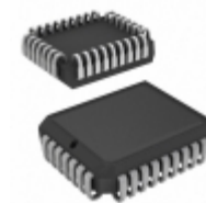
CY7C4241-15JXCT Cypress Semiconductor Corp IC SYNC FIFO MEM 4KX9 32-PLCC
