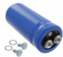
CGS752U040R4C Cornell Dubilier Electronics (CDE) CAP ALUM 7500UF 40V SCREW
