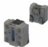
3313J-1-501E Bourns, Inc. TRIMMER 500OHM 0.125W J LEAD TOP
