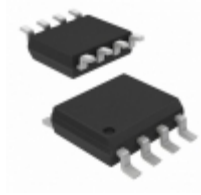
IRF7463TRPBF International Rectifier (Infineon Technologies) MOSFET N-CH 30V 14A 8-SOIC
