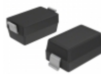
BZT52C20-G3-18 Vishay Semiconductor Diodes Division DIODE ZENER 20V 410MW SOD123
