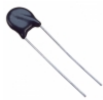
ERZ-V10D361 Panasonic Electronic Components VARISTOR 360V 3.5KA DISC 10MM
