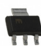
MIC2920A-12BS Microchip Technology IC REG LDO 12V 0.4A SOT223
