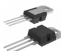
MIC2920A-12BT Microchip Technology IC REG LDO 12V 0.4A TO220-3
