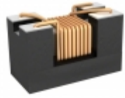
DLW31SN601SQ2L Murata Electronics CMC 260MA 2LN 600 OHM SMD
