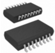
ADUM4400WARWZ ADI (Analog Devices, Inc.) DGTL ISO 5KV 4CH GEN PURP 16SOIC
