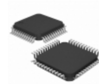
S9S12GA128F0VLF NXP Semiconductors / Freescale 16-BIT MCU S12 CORE 128KB FLAS
