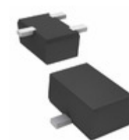
2SB1218G0L Panasonic Electronic Components TRANS PNP 45V 0.1A SMINI-3
