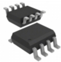
AD7390ARZ Analog Devices Inc. IC DAC 12BIT 3V SRL-IN 8-SOIC
