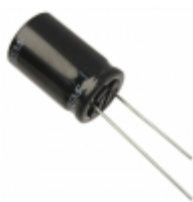
EEU-FR1V222B Panasonic Electronic Components CAP ALUM 2200UF 20% 35V RADIAL
