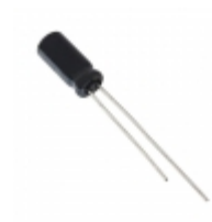
EEU-FR1V330B Panasonic Electronic Components CAP ALUM 33UF 20% 35V RADIAL
