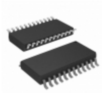
AD8403AR100 ADI (Analog Devices, Inc.) IC DGTL POT 8BIT 100K 4CH 24SOIC
