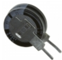
DXJ-5R5V224U Elna America CAP 220MF -20% +80% 5.5V T/H
