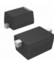
CMOZ15L TR Central Semiconductor Corp DIODE ZENER 15V 250MW SOD523
