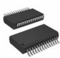
PIC16LF1903-I/SS Microchip Technology IC MCU 8BIT 7KB FLASH 28SSOP
