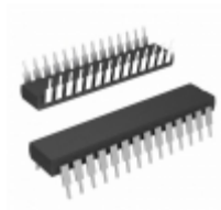
PIC16LF1903-I/SP Microchip Technology IC MCU 8BIT 7KB FLASH 28SDIP
