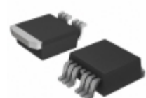
IXTA160N075T7 IXYS MOSFET N-CH 75V 160A TO-263-7
