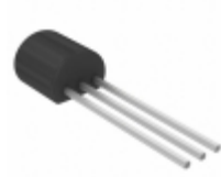
BC556B_J18Z AMI Semiconductor / ON Semiconductor TRANS PNP 65V 0.1A TO-92
