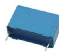
B32523Q3335J000 EPCOS CAP FILM 3.3UF 5% 250VDC RADIAL
