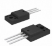
FQPF9N30 AMI Semiconductor / ON Semiconductor MOSFET N-CH 300V 6A TO-220F
