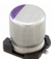
2R5SVPC180MY Panasonic Electronic Components CAP ALUM POLY 180UF 20% 2.5V SMD
