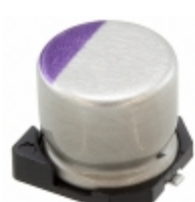
2R5SVPC390M Panasonic Electronic Components CAP ALUM POLY 390UF 20% 2.5V SMD
