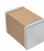
CL21F475ZOFNNNG Samsung Electro-Mechanics America, Inc. CAP CER 4.7UF 16V Y5V 0805
