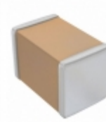
CL21F475ZPFNNNG Samsung Electro-Mechanics America, Inc. CAP CER 4.7UF 10V Y5V 0805
