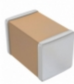
CL21F475ZOFNNNE Samsung Electro-Mechanics America, Inc. CAP CER 4.7UF 16V Y5V 0805
