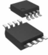
MAX4017EUA+T Maxim Integrated IC OPAMP BUFFER 200MHZ RRO 8UMAX
