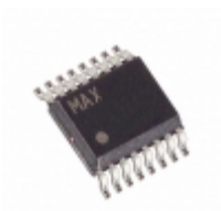
MAX4018EEE Maxim Integrated IC OPAMP TRIPLE R-R HS 16-QSOP
