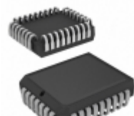
AT49LH00B4-33JX Microchip Technology IC FLASH 4MBIT 33MHZ 32PLCC
