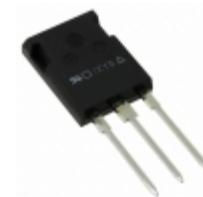
IXER60N120 IXYS IGBT 1200V 95A 375W ISOPLUS247
