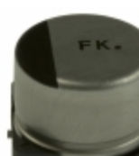
EEE-FK1A331AP Panasonic Electronic Components CAP ALUM 330UF 20% 10V SMD
