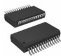
PIC24FJ16MC102-I/SS Microchip Technology IC MCU 16BIT 16KB FLASH 28SSOP
