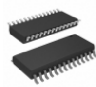
PIC24FJ16MC102-I/SO Microchip Technology IC MCU 16BIT 16KB FLASH 28SOIC
