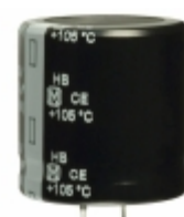
ECO-S2WB271EA Panasonic Electronic Components CAP ALUM 270UF 20% 450V SNAP
